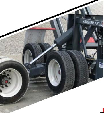
Hydraulically operated "pushdown" axles lift the machine to allow quick and easy movement of the machine without the need to move the main axle from radial to transport mode.
